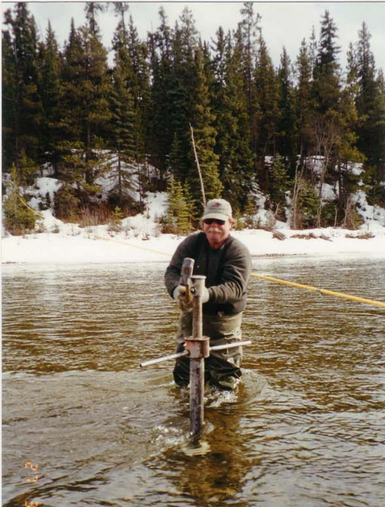
Photo B-1. Grinding outer barrel into substrate.
