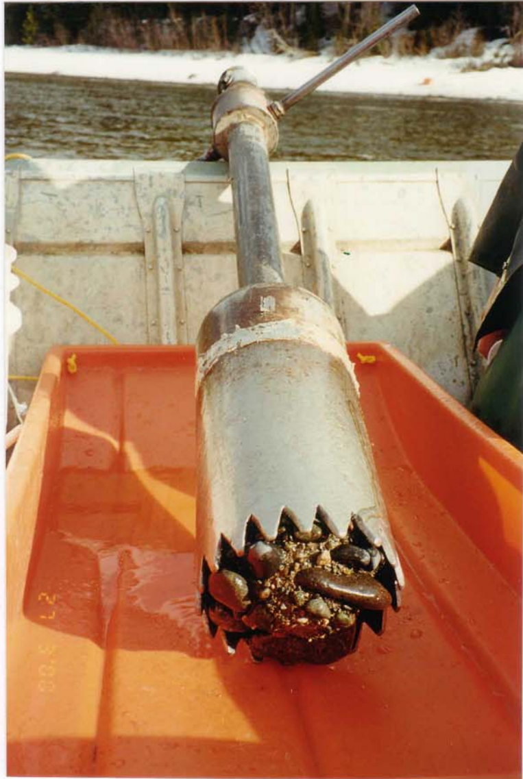
Photo B-7. Close-up of sampler containing frozen substrate sample.
