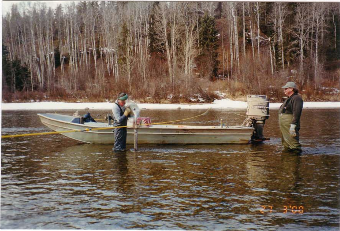
Photo B-5. Boat moored to a tagline to serve as an instream working platform.
