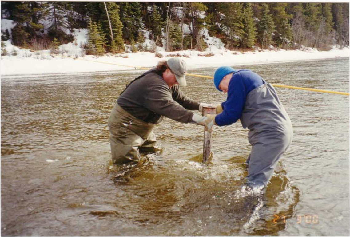
Photo B-1. Grinding outer barrel into substrate.
