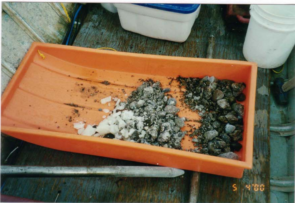
Photo B-9. Sample split into top and bottom halves.
