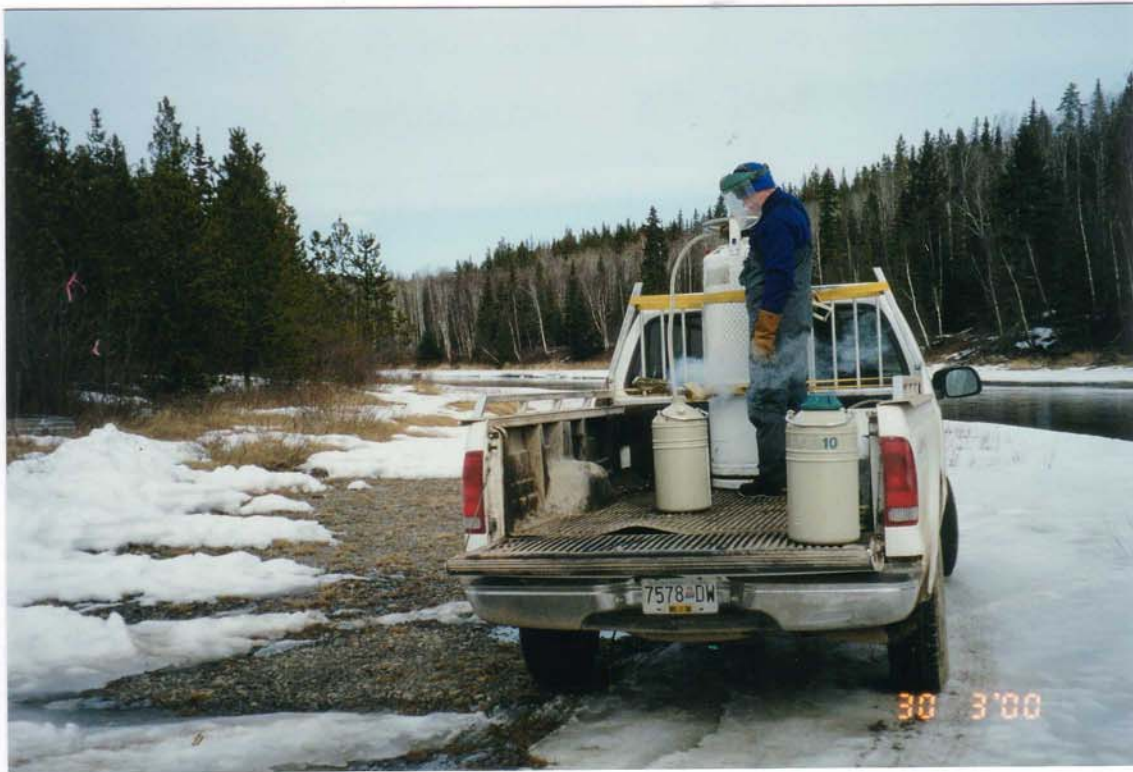
Photo B-3. Filling Dewar flasks with liquid nitrogen.
